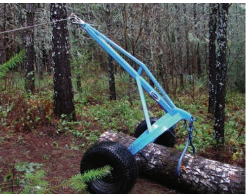
Figure 11. Arches attached to winch cables can be used to lift the front end of logs when the winch cable is drawn tight facilitating movement of the log back to the winch.
