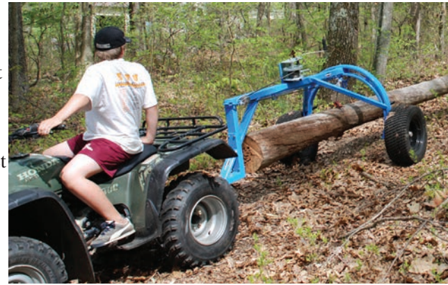
Figure 3. Arches are arguably the safest and most efficient way to move larger logs with four wheelers.
