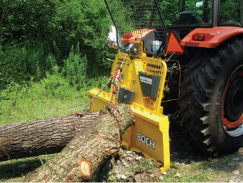
10 a. Figure 10. Skidding winches provide a safe means of using farm tractors. The logs are first pulled to the winch using cables (a) and then lifted off the ground and skidded from the woods (b).
