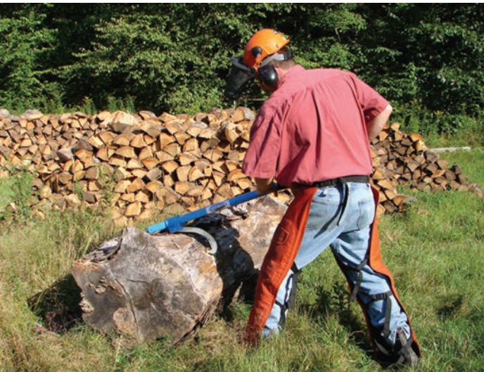
Figure 2. Cant hooks and Peaveys are valuable tools to help move logs by hand.
