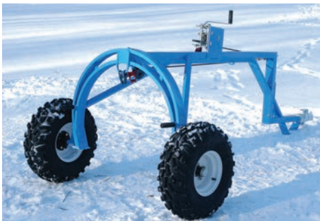
Figure 7. Arch with a hand operated winch with cable that attaches to chains wrapped around logs.
