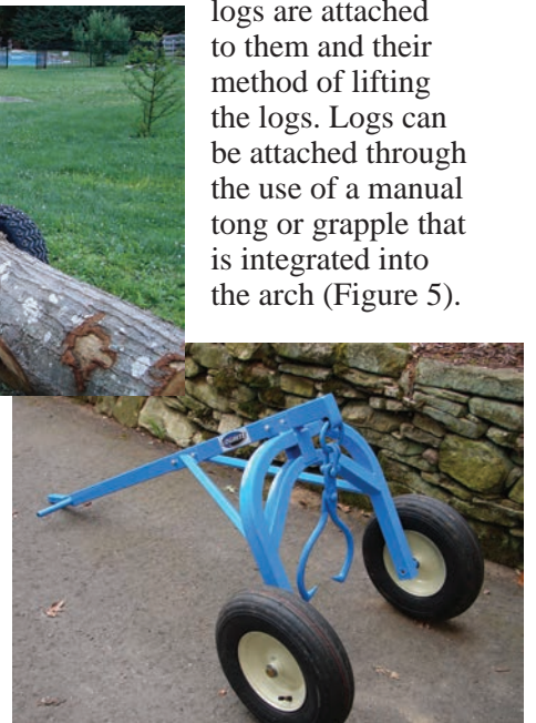
Figure 5. Some arches use tongs to grab logs while others use cables and chains.
